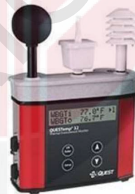
Figure 32: QUESTemp o36 WBGT Thermal Environmental Monitor Source: (QUEST Technologies, 2008)
