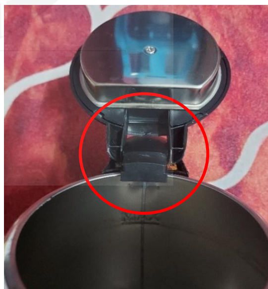
Figure 5.4: Plastic parts in stainless steel electric kettle F
