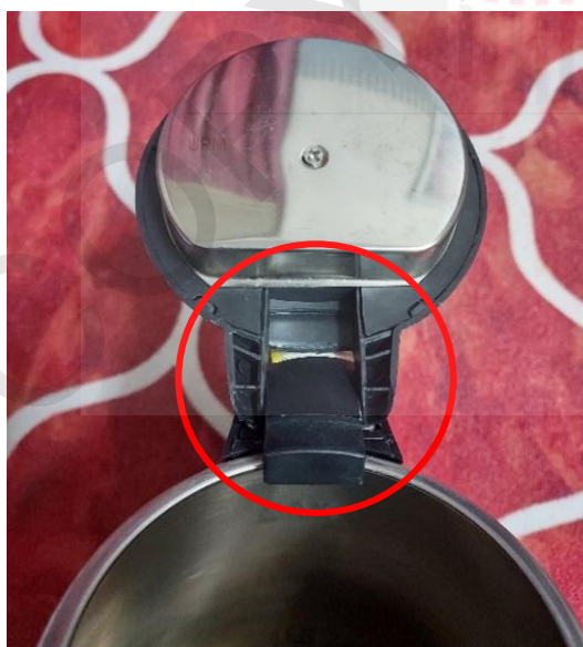
Figure 5.3: Plastic parts in stainless steel electric kettle E
