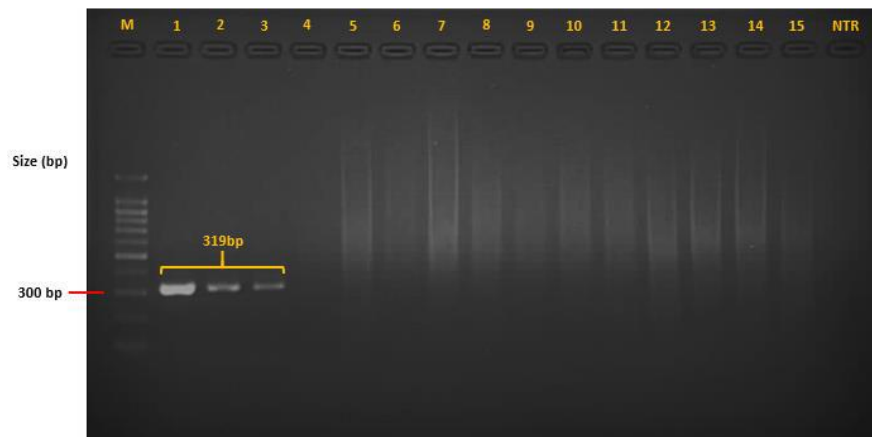
Figure 4.2 PCR assay for detection of NoV RdRp gene in porcine faecal samples by using universal primer pair p290/p289 to produce 319 bp PCR band. Electrophoresis was carried out on 2.0% (w/v) agarose gel. All samples show no significant amplification
