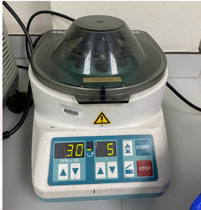
Figure 11: The Hettich® EBA 20 centrifuge machine set at 3000 rpm for 5 minutes to separate plasma from red blood cells
