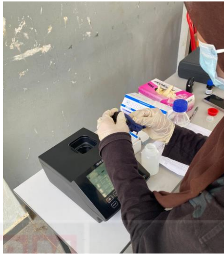
Hanna instrument HI801-02 iris Visible Spectrophotometer for iron analysis
