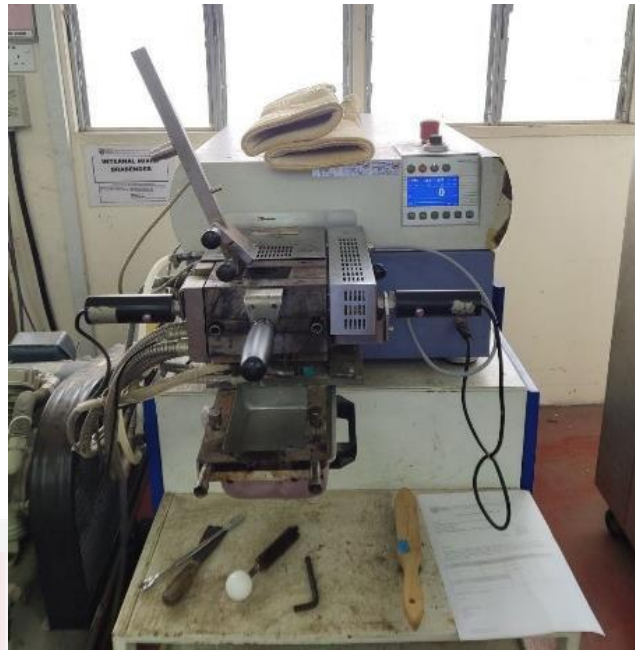
Figure 3.4: HAAKE Melt Blending machine used to mixing the PET and CNTs for fabrication of PET nanocomposite.
