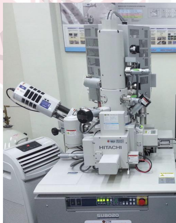
Figure 2.7: Field Emission Scanning Electron Microscopy Machine for determination of surface morphology (UPM, 2020).
