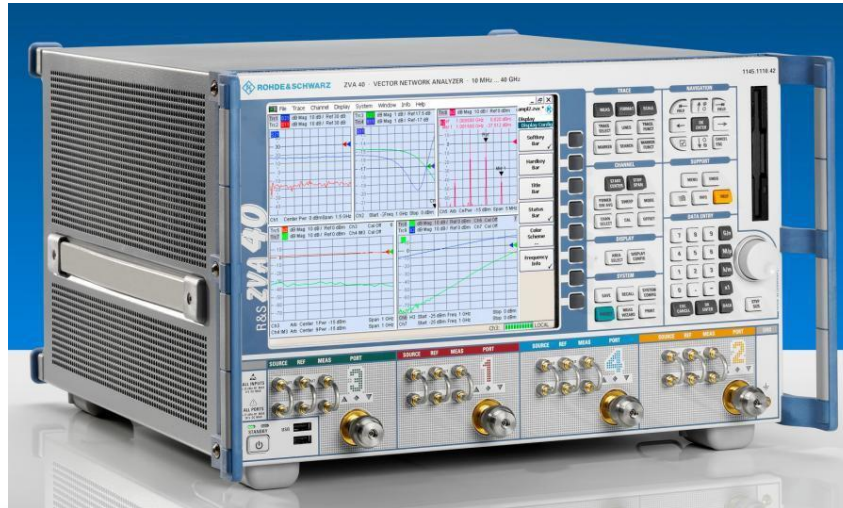
Figure 2.8: Vector Network Analyzer (VNA) Machine to observe the EMI absorbance properties (UPM, 2021).
