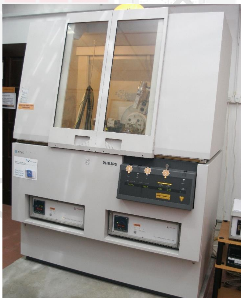
Figure 3.8: XRD instrument model PANalytical PRO PW3040 that been use in this study.
