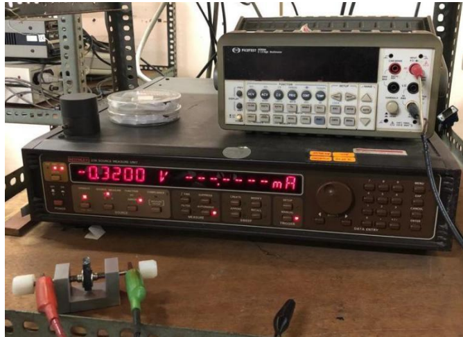
Figure 3.12: The electrical conductivity was conducted using two-point probe method (UPM, 2021).
