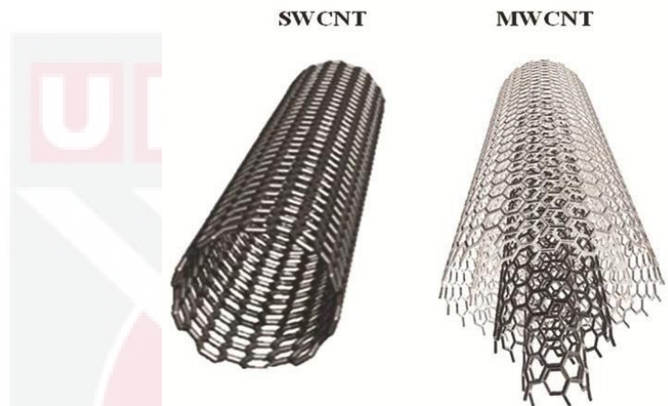
Figure 2.4: Structure of Single-walled Carbon Nanotubes (SWCNT) and Multi-walled Nanotubes (MWCNTs) (Choudhary & Gupt, 2011).
