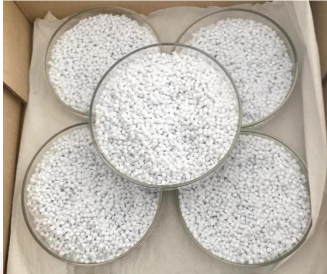
Figure 3.3: The PET sample were divided to several parts inside the petri dish for drying process.
