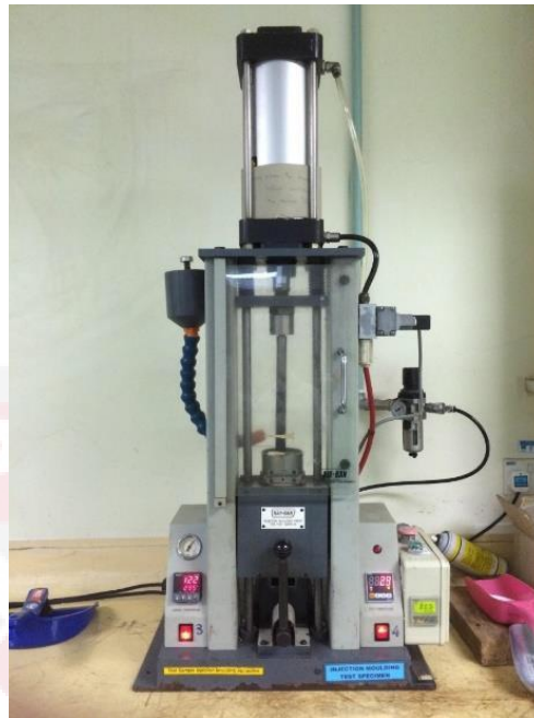
Figure 3.5: The injection molding method were conducted using Ray Ran Injection Molding Press.
