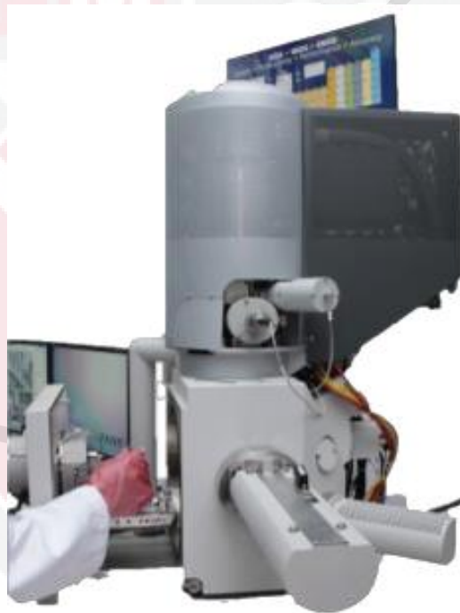
Figure 3.9: FESEM instrument model that been used in this study (ITMA, 2021).
