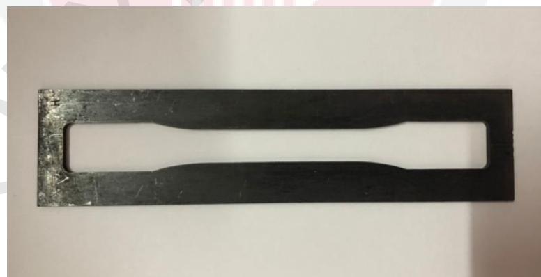
Figure 3.6: All the sample are casting using dog bone mold.
