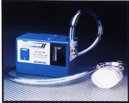
Figure 3.3 : Gillian Air Pump Sampling model
