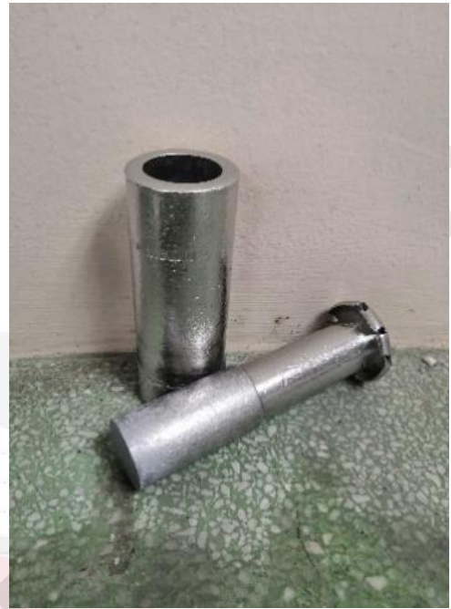
Figure 3.3: Plunging apparatus used for crushing ASF glass frits
