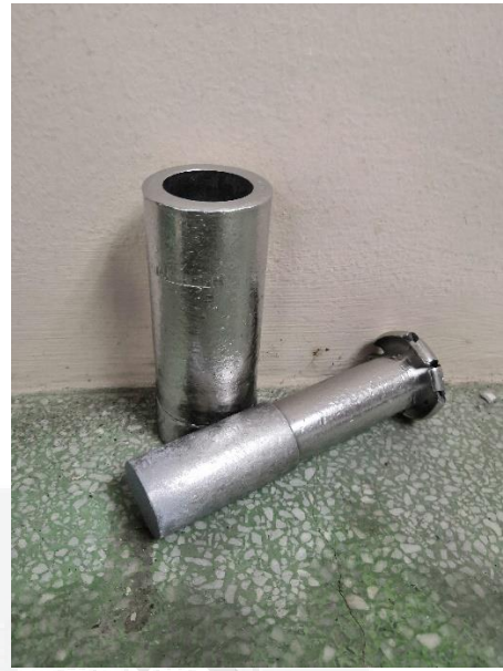
Crushing using plunger from ASF glass frits
