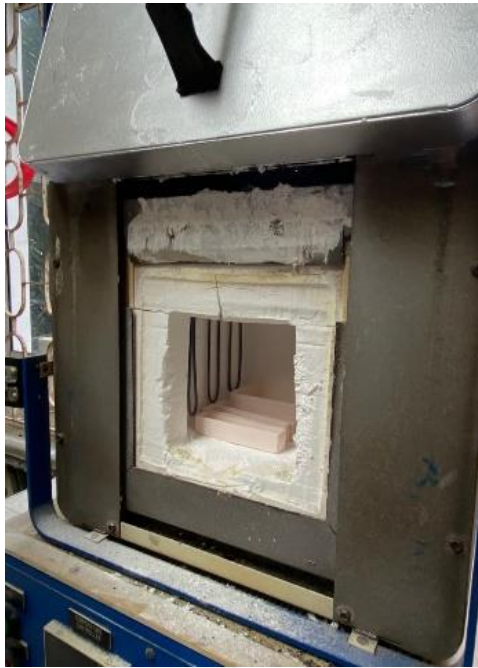
Figure 3.2: Electrical furnace for melting process
