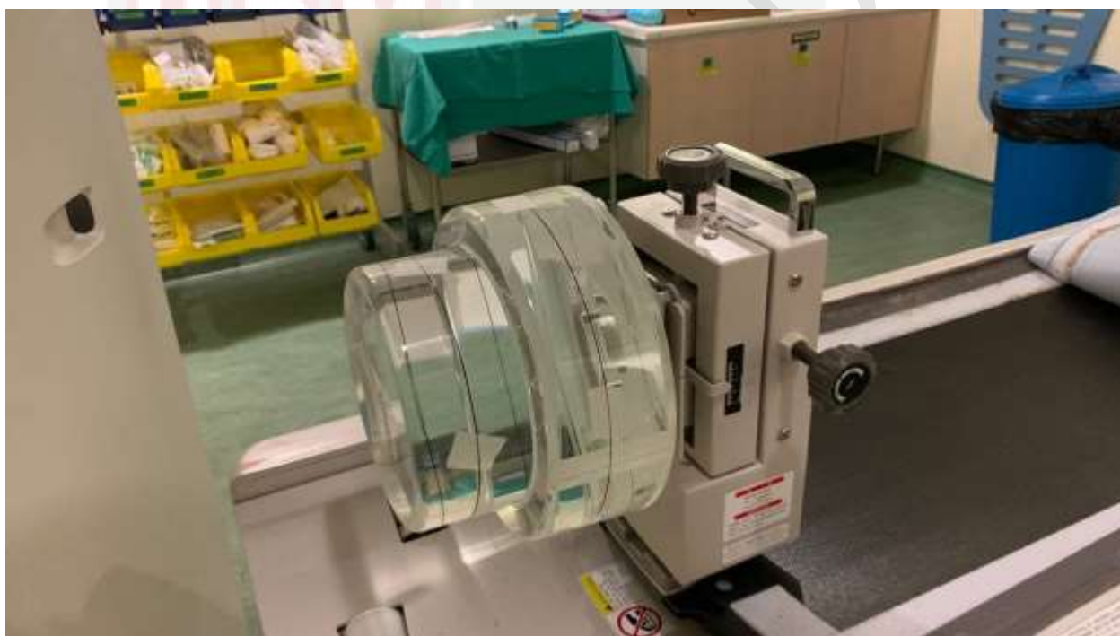
Figure 3.1 Water phantom placed on holder before calibrated
