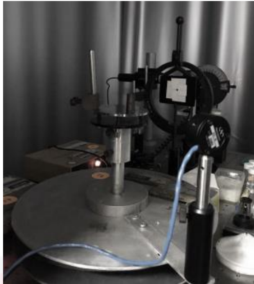
Figure 3.14 Experimental setup of SPR located at Applied Optics Laboratory, Physics Department, Faculty of Science
