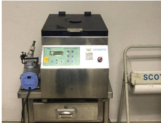
Figure 3.5 Spin coating machine
