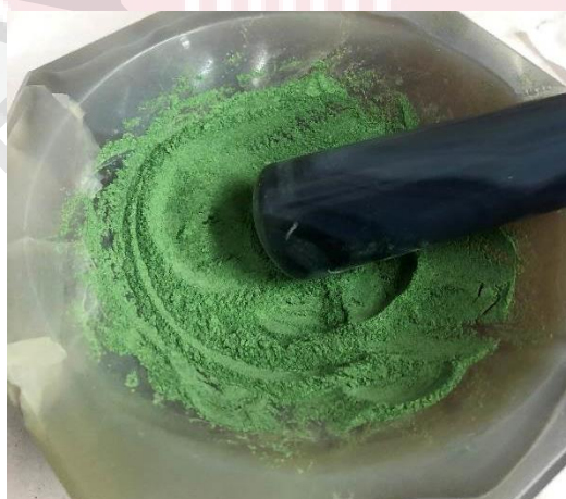
Figure 3.5: The light green fine powder obtained after the grinding process.
