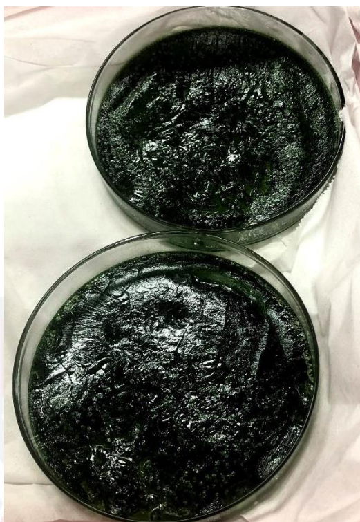
Figure 3.4: The dark green powder obtained after the drying process was undergone in the oven at 110 °C for 24 hours.
