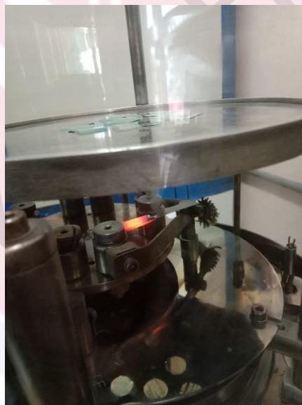
Figure 3.6: The tungsten boat filled with 15 mg of F_{16}CuPc powder was heated up.
