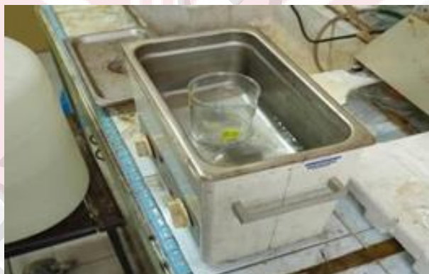
Figure 3.2: The glass substrates were sonically cleaned by ultrasonic cleaner for 10 mins.
