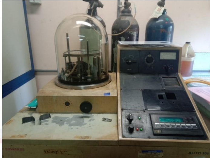
Figure 3.3: Edward Auto 306 thermal evaporator.
