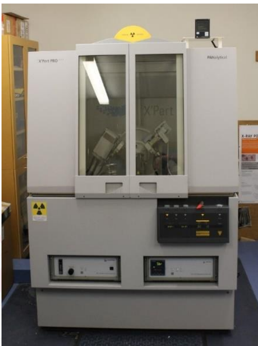
Figure 3.11: The XRD spectrometer used to identify the structural properties of F_{16}CuPc thin films.
