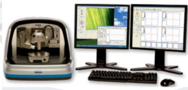
Figure 3.12: AFM spectrometer used to observe the morphological properties of F_{16}CuPc thin films.
