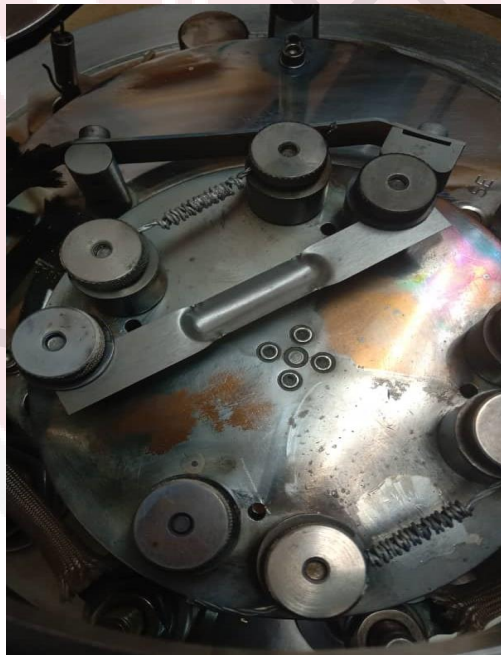
Figure 3.4: The tungsten boat was placed for the thermal deposition process.
