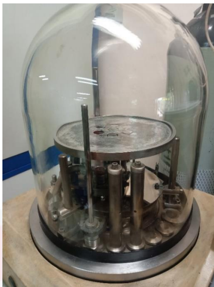
Figure 3.5: The glass substrates were placed on the substrates holder.
