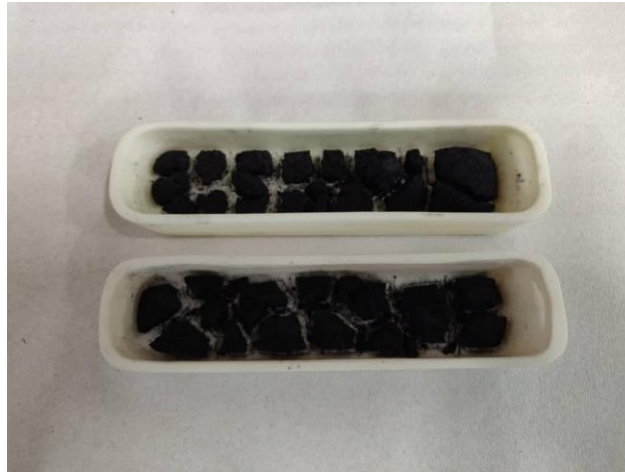
Figure 3.7(a): Sample after calcine at 500°C for 5 hours
