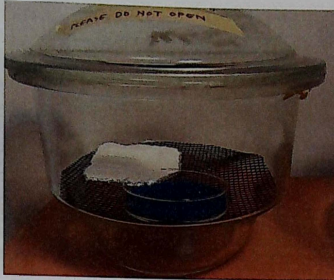
Figure 3.7: Silica gel was placed in desiccator with a sample
