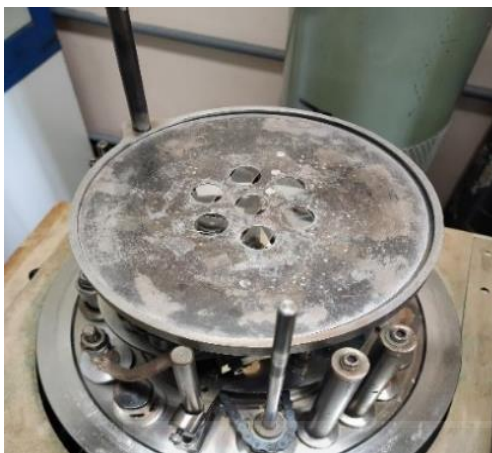
Figure 3.4 (a): Masker used for thermal evaporation technique
