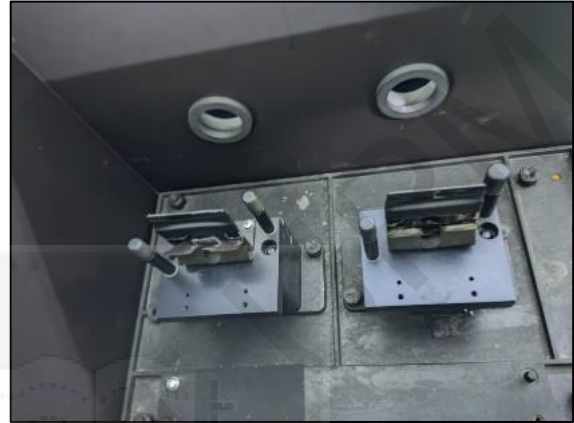
Figure 3.9 (b): reference and sample holders of the spectrophotometer
