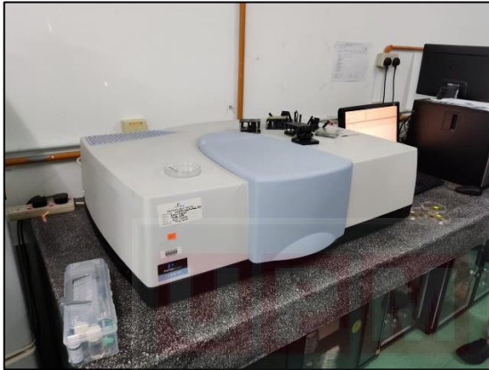
Figure 3.9 (a): UV/visible/NIR spectrophotometer Perkin Elmer model Lambda 750
