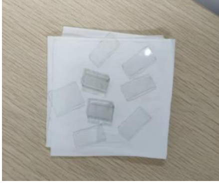
Figure 3.1 (a): Fixed size glass substrate after being cut
