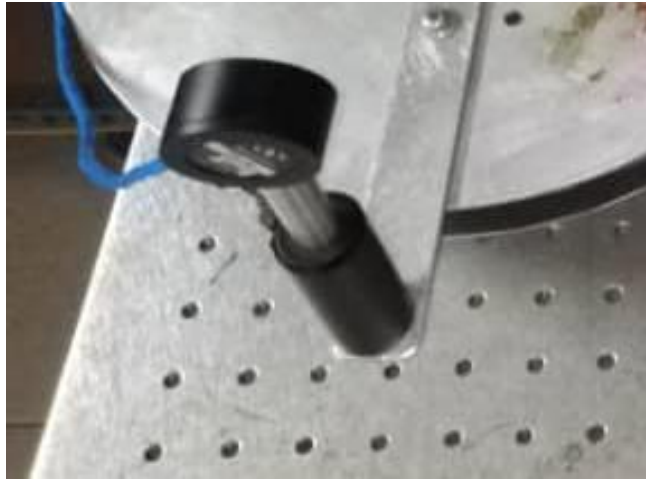
Figure 3.5: Photodiode used to detect the reflected light.
