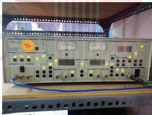
Figure 3.7: Example of lock-in amplifier used in SPR setup.
