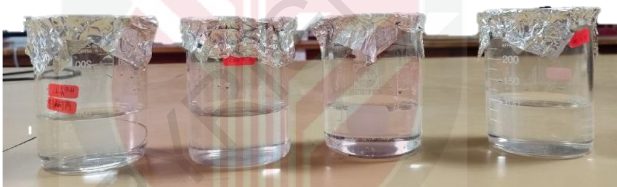
Figure 3.6 The chemical bath deposition (CBD) solution.
