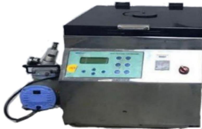
Figure 3.4 Spin coater machine.
