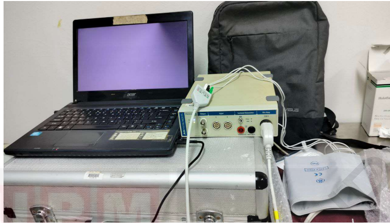
Figure 3.4: Recording of EEG Using Powerlab 26T Data Acquisition System Hardware (ADInstruments Pty Ltd).
