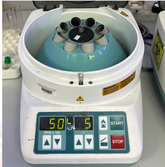
Figure 3. Blood samples stored in red plain tubes were centrifuged at 5000 rpm for 5 minutes.
