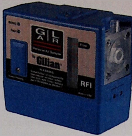
Figure 3.4.2: Gilian GilAir-3 Air Sampling Pump (Source: Sensidyne)
