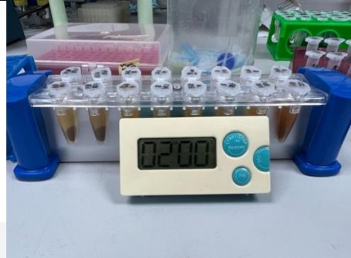
Magnetic separator rack for DNA extraction using magnetic beads kit
