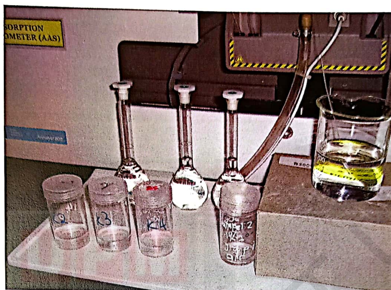
Figure C1: Determine the metal concentration using air-acetylene Perkin-Elmer™ flame atomic absorption spectrophotometer(AAS)
