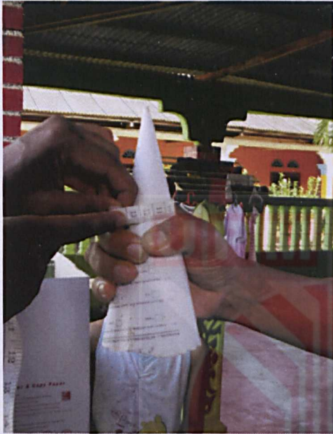
Figure 1: Measuring respondent's internal grip circumference
