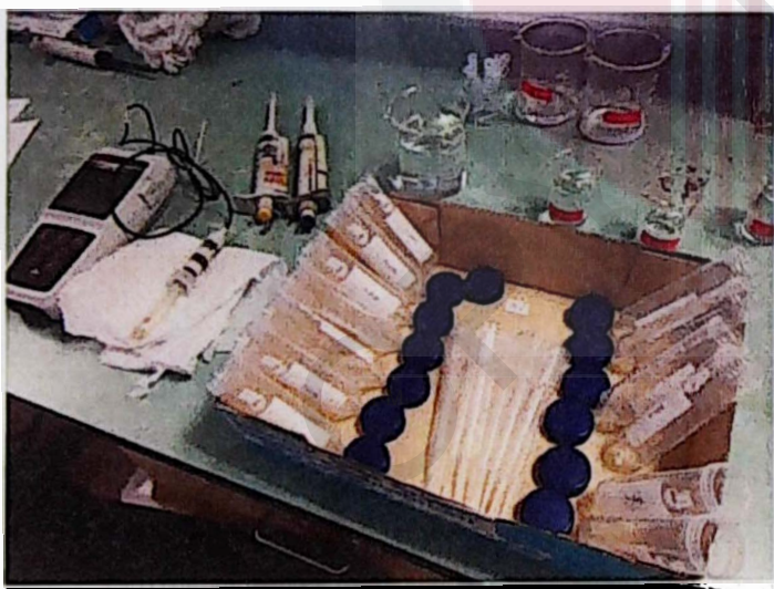
Figure 3.4.3.5 : pH meter used to adjust the pH and the labelled tubes to transfer in every phase
