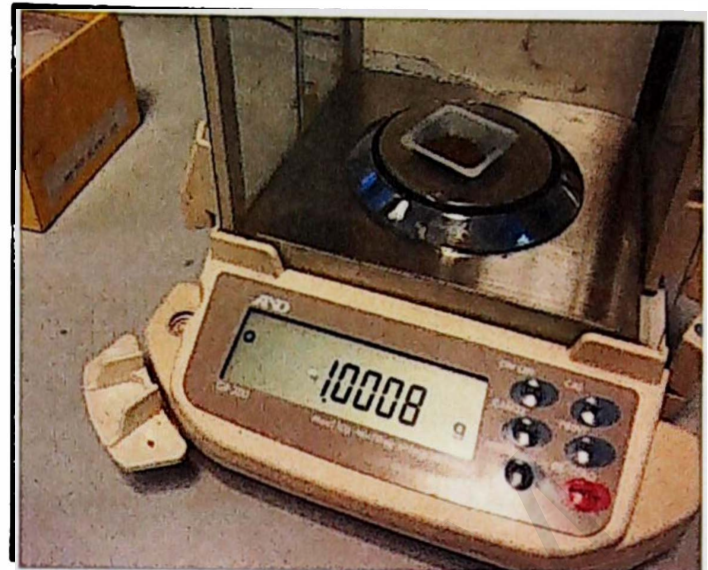
Figure 3.4.2.3 : Soil samples were weighed carefully to 1g
