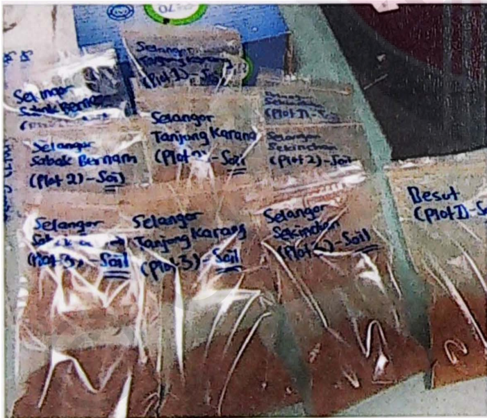
Figure 3.4.1.5 : Paddy soil samples after air-dried and homogenized
