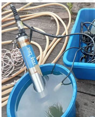
Multiparameter reading in the water sample of crayfish rearing tank
