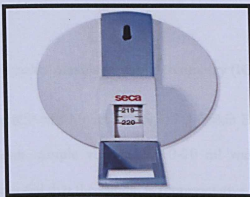
Figure 3.5: Portable Seca body meter which was used to measure height of respondents
