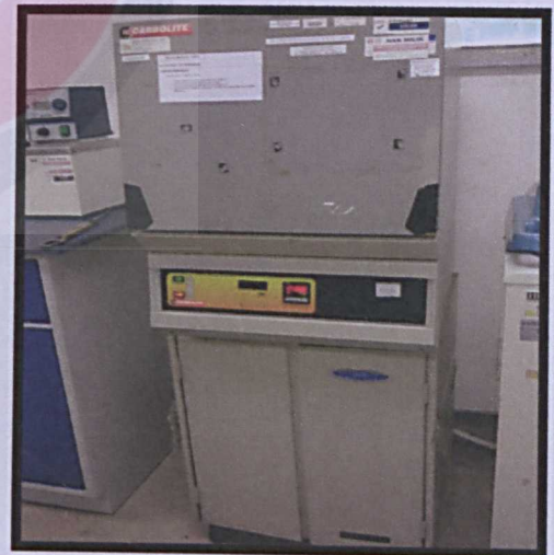
Figure 3.8: Sample was placed in a preheated muffle furnace at 200–250 °C for 30 min. Then, sample was ashed for 4 h at 480 °C. 2 ml of concentrated HCl was added and the sample was evaporated to dryness, removed. 5 ml of 2 M HCl was added and the tube was again swirled. Continued.
