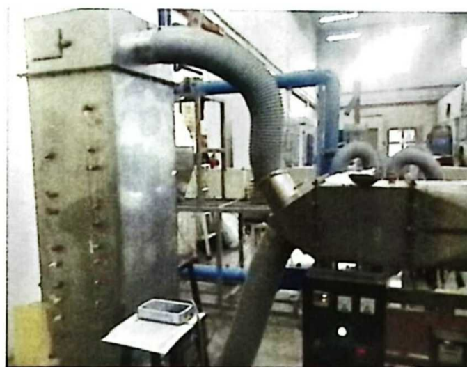
Figure 3.6: Inline Paddy Dryer
