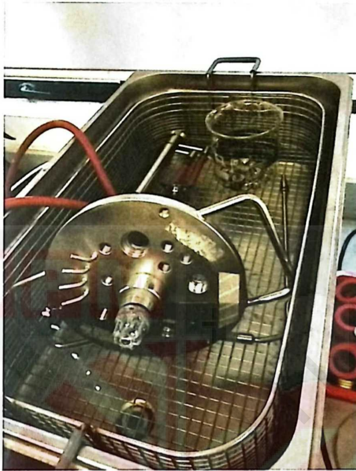
Top plate of jacketed glass vessel and other small parts in a sonicator bath for clean purposes
