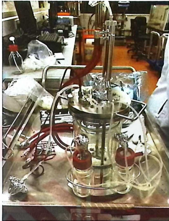
Side view of jacketed glass vessel
