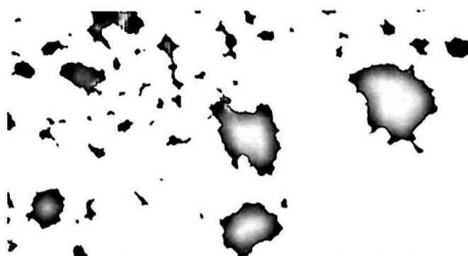
Appendix B14: Image analysis for determination of particle size of CFO
