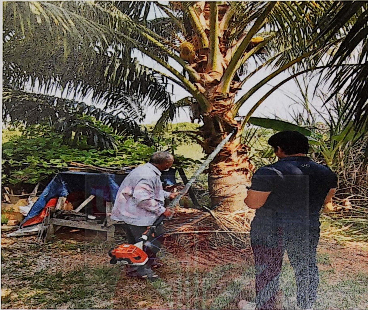
Figure 3.2 Measurement of vibration using HVM 100 with tri-accelerometer attached to the Cantas machine
