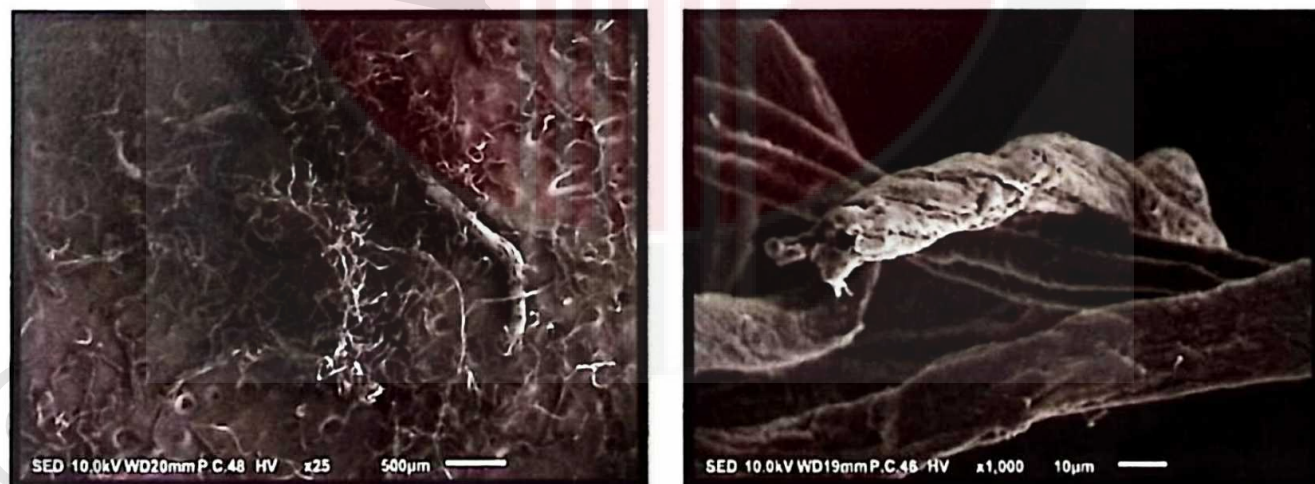
Figure 4. 12: SEM micrographs of treated durian husk cellulose fiber at 500x (left) and 1000x (right) magnification.
