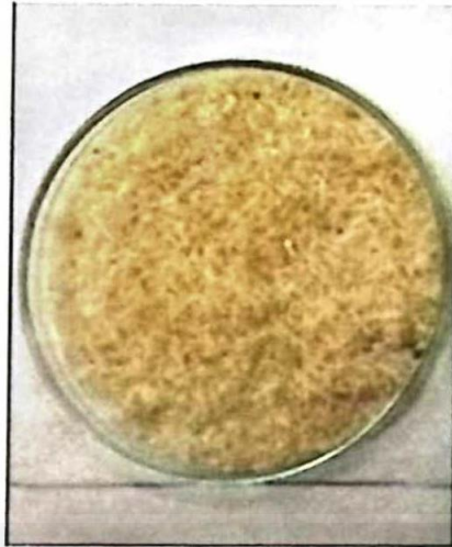
Figure 21: Top view of dried desiccated coconut by Microwave oven (440W)
