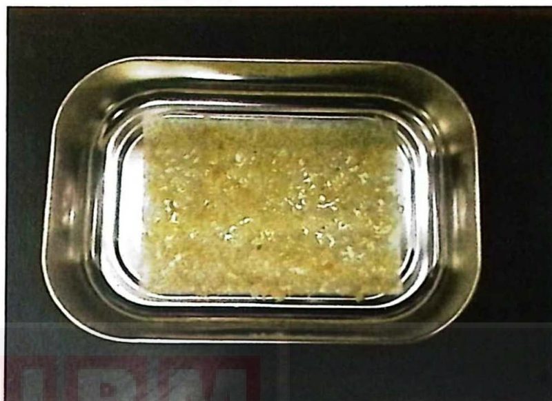
Figure 27: Dried desiccated coconut was distributed evenly on the blotting paper in a drying tray for measuring the surface oil content.
