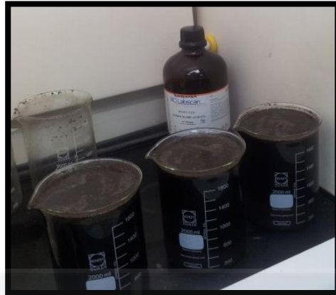
Figure 6 Demineralization process of HC treated with 5 litres of 1M HCl for 24 hours.
