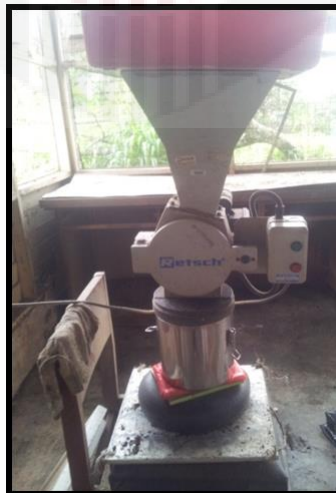
Figure 5 Grinder machine used to grind the HC into meal form
