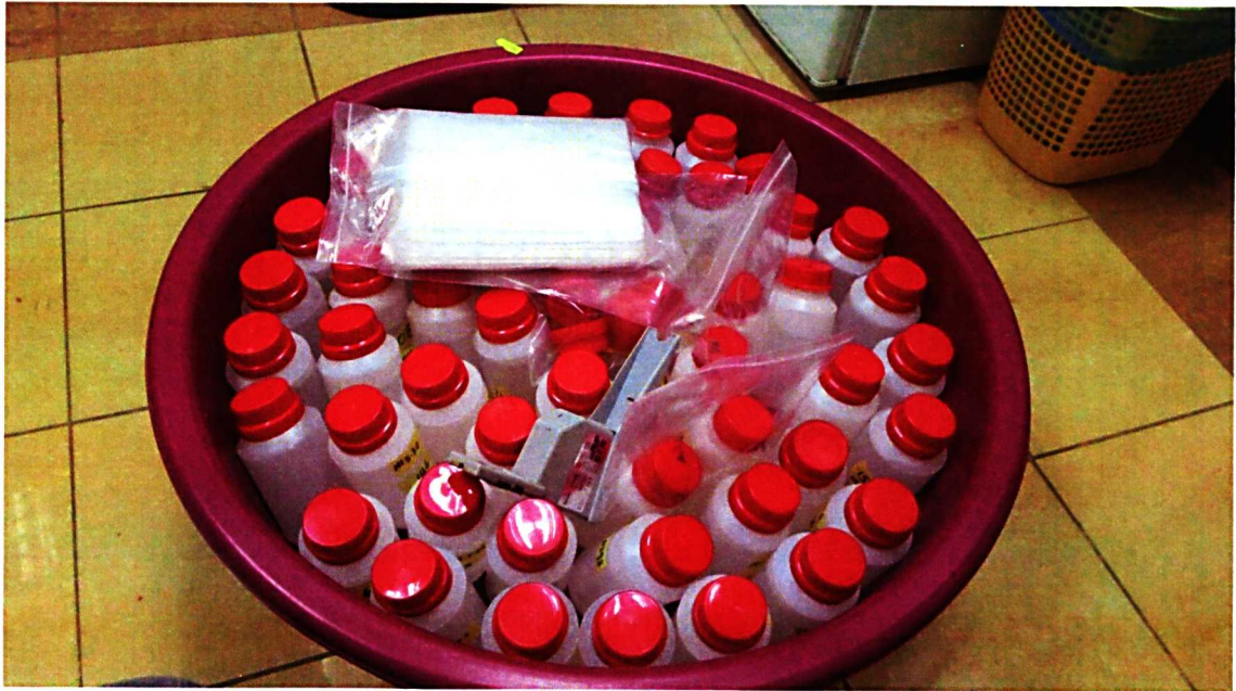
HDPE bottles that had been washed with nitric acid, labeled and filled with water samples.
