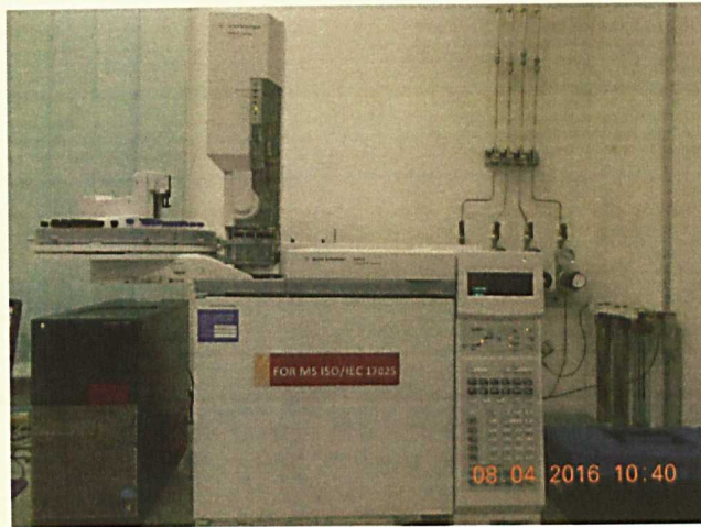
Figure 3.1: Gas-chromatography equipped with FID
