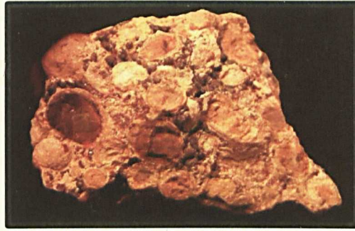
Figure 2.2 : Bauxite or Al Hydrates, an elementary ore of Al (Harder, 2015)
