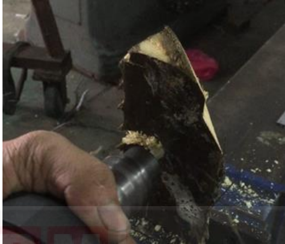
Figure 4.1-12: Cutting OPF Using Small Straight Router Bit
