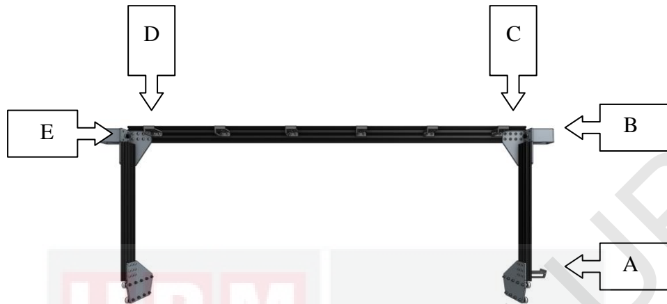
Figure 11 : Gantry Positioning completely assemble
