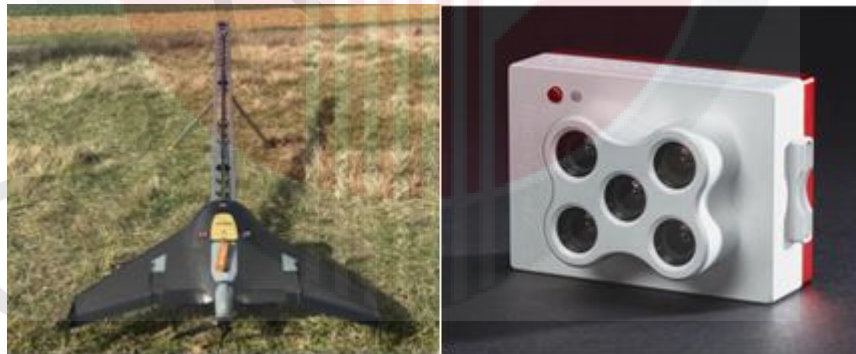
Figure 3. 3 UAV UX5AG and Red-Edge multispectral camera
