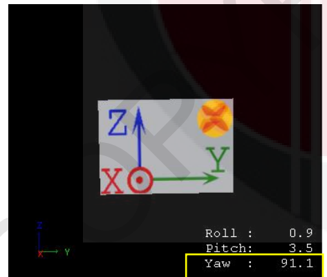
Figure 4.6: IMU sensor orientation when yaw motion data is positive
