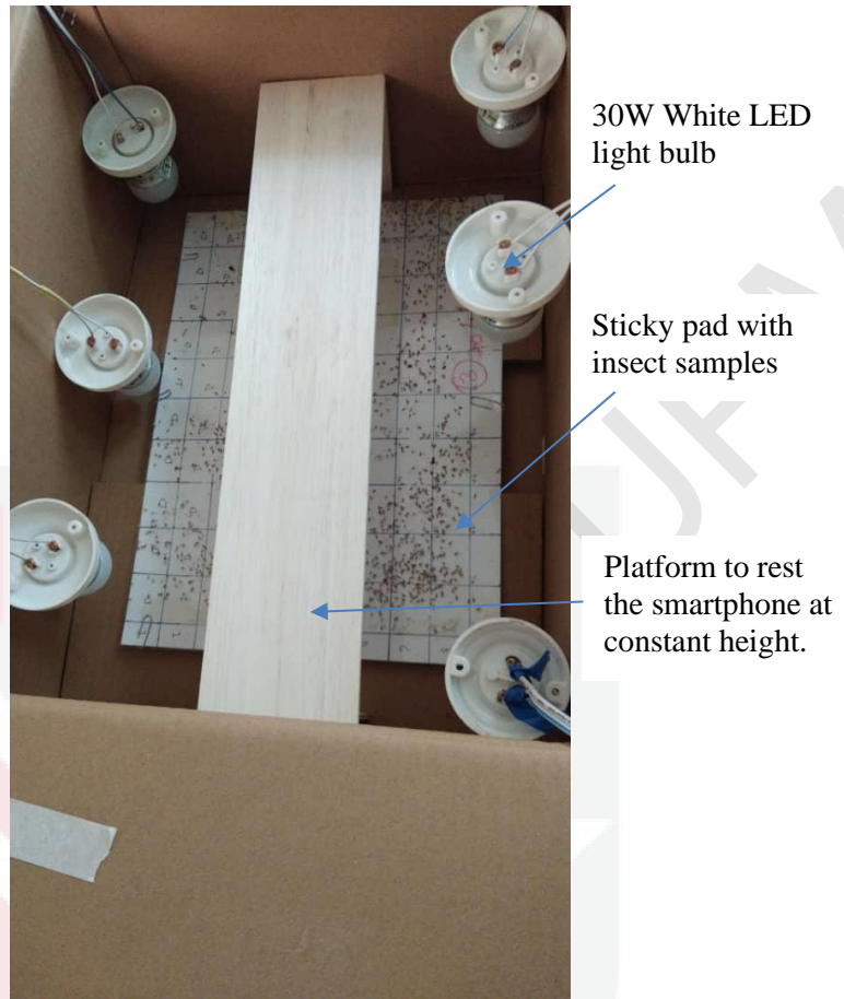
Figure 3.6 The image acquisition setup to collect the insect pest image.
