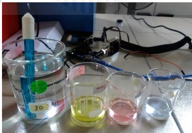
Figure 12: Apparatus for pH Sensor calibration
