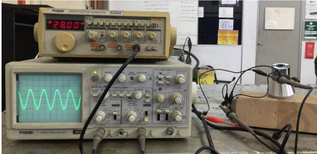
Figure 18: Horn tuning set up with bare transducer
