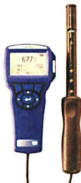
Figure 5: TSI Q-Trak™ Indoor Air Quality Monitor 7575 (Source: TSI Website)
