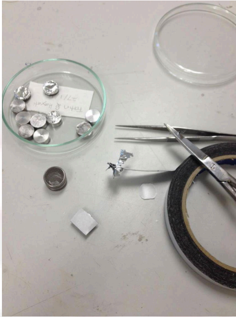
Figure 3.1: Mounting process was done by sticking the sample onto the stub using double sided tape and coating with gold coat in sputter coater.
