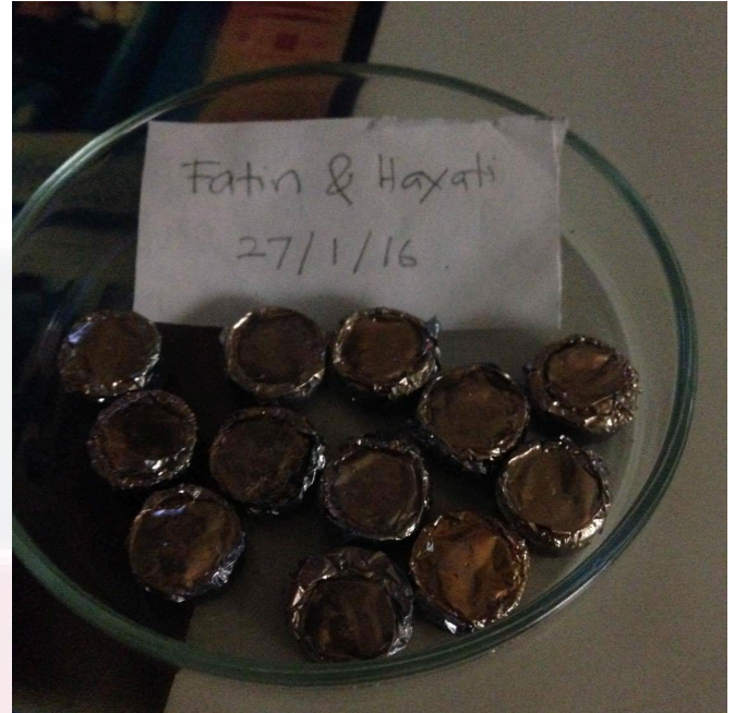
Figure 3.2: Sample after coating with gold coat in sputter coater.
