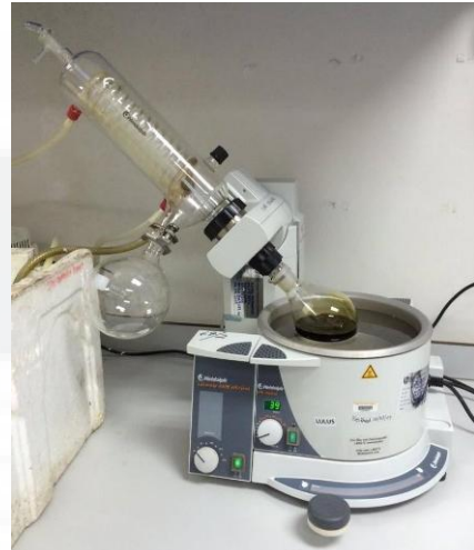
Figure 8.3.6 Filtrate evaporated using Rotary Evaporator at 40°C
