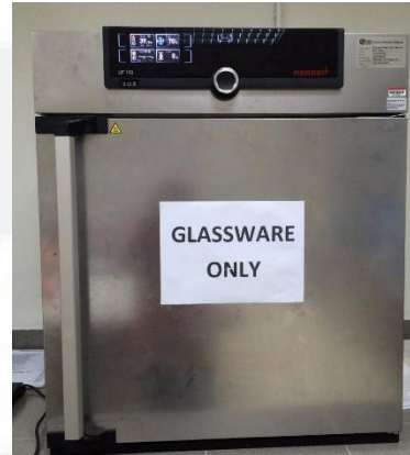
Figure 8.3.2 Hot dry oven to keep the leaves until the leaves crisp and the weight even
