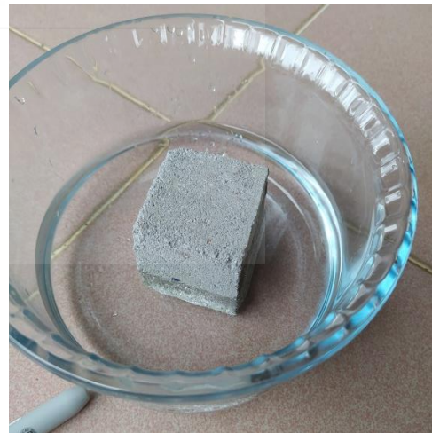
Figure 3.6.2: Distilled water was put until it reached the mark
