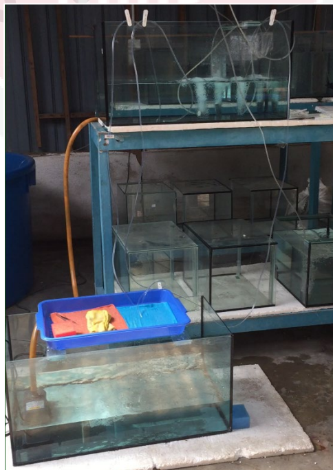
Photograph of recirculation anaesthesia delivery system for Goldfish surgery
